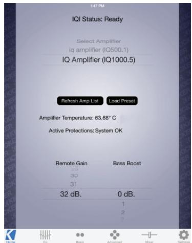
The 'HOME' screen will display all connected IQ amps, their operating temperature, remote gain and bass boost settings. Use the 'Load Preset' button to apply a previously configured preset to the IQ amplifier that is currently selected.
