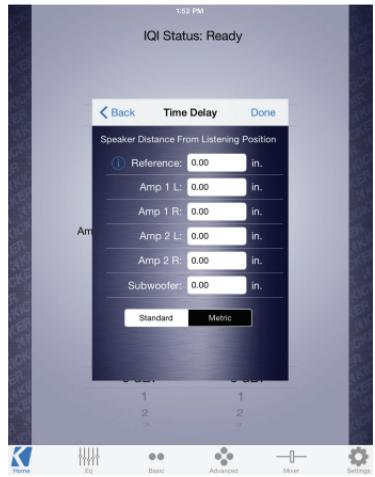
Set the distance of each speaker from the primary listening position. This will automatically configure the correct time-delay for each speaker to present the best sound-stage. The Reference Speaker setting should be set if there is a speaker in use that is not connected to the IQ amplifier currently being configured, and whose speaker is farthest from the listening position.
