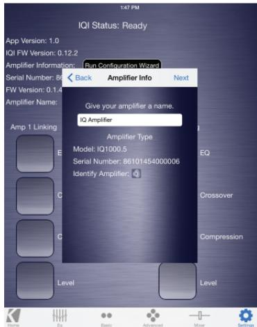
TWEEQ will scan and identify all connected amplifiers. KICKER has support for multi-amp installations using the IQI accessory. You may toggle between amps from the 'HOME' screen.
