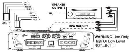
The use of twisted pair interconnects is recommended for all installations to minimize noise. When routing these cables through the automobile, try to keep them away from factory wiring harnesses and other power wiring. If you need to cross any of this wiring do so at a 90 degree angle to reduce the potential of noise problems.
