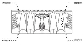
With the shroud removed, you now have access to the four mounting holes in the mounting feet and all wiring connections. Drill 4 holes using a 7/64" drill bit and use the supplied #8 screws to mount the amplifier.
