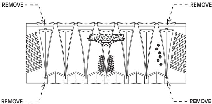
With the shroud removed, you now have access to the four mounting holes in the mounting feet and all wiring connections. Drill 4 holes using a 7/64" drill bit and use the supplied #8 screws to mount the amplifier.
