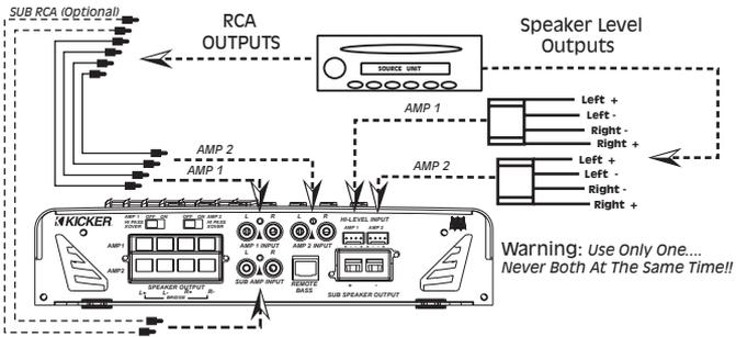
When using both sets of High Level inputs on the KX700.5, the supplied RCA dummy plugs must be inserted into the AMP 2 inputs in order for the fader to work properly. If the amplifier is being used in any other configuration DO NOT USE THE RCA DUMMY PLUGS!
