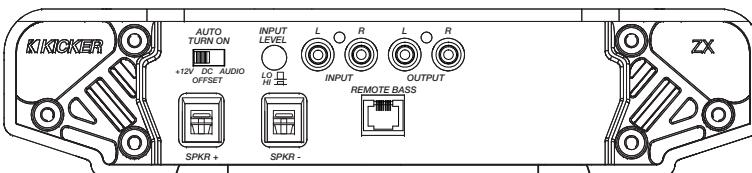
**1. Automatic Turn-On Selection** The ZX series offers three different automatic turn-on modes that can be selected on the end panel; +12V, DC Offset, and Audio. Using either the DC Offset or Audio mode causes the REM terminal to have +12V out for turning on additional amplifiers.
