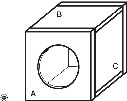
**Sealed Enclosures:** The KM subwoofer generates more sound pressure than competing marine subwoofers on the market and excels when used in sealed boxes. These sealed enclosure designs give the smoothest response with increased energy at the lowest frequencies, 20 to 40Hz, delivering massive amounts of highly-accurate bass.
