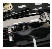
8. Drill a 3/4" hole in each bag as pictured and install the supplied rubber gromets.
