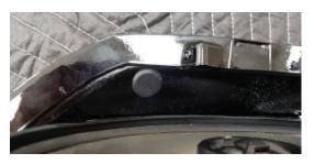
6. Install the supplied grilles to the lids using the supplied screws.
