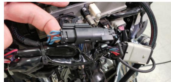
2. Plug the 4-pin connector into the front kit's rear inputs, then route the RH14HDT harness through the neck and wiring track to the rear of the bike .
