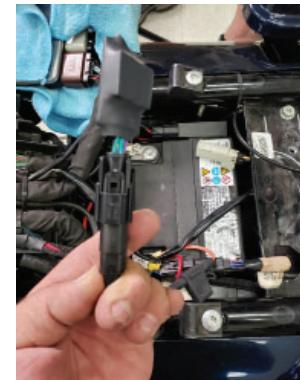
4. Find the rear speaker 4-pin plug and unplug the resistor pack.
