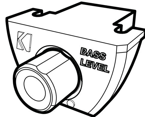
With the CXARC remote bass level control, you have the ability to control the output level of the amplifier remotely. To surface-mount the CXARC remote bass level control, simply screw the remote to the chosen location, then run the cable from the controller to the "Remote Bass" jack on the amplifier panel. Do **NOT** connect/disconnect while the amplifier is on. Connecting the 3.5mm cable without the remote will cause the amplifier to output at full gain, possibly damaging your speakers.
