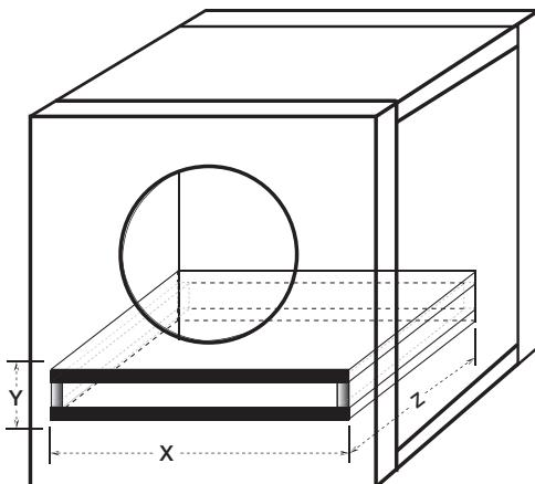
The displacement of the port must be calculated and added to the internal volume of the final design. The dimensions for X, Y, and Z may vary based on the thickness of the material used to make the port.
