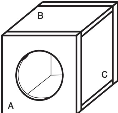
**Sealed Enclosures:** These sealed enclosure designs give the smoothest response with increased energy at the lowest frequencies, 20 to 40Hz, delivering massive amounts of highly-accurate bass.
