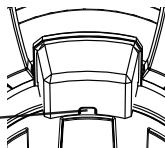
**Infinite Baffle Mounting:** The infinite baffle mounting method effectively utilizes the storage space of most boats. Use caution when mounting speakers through any panel of the boat. Please be aware of wiring harnesses, springs, hinges, and folding seat mechanisms that may interfere with the operation of the boat or speaker system. Mark the panel for the hole cut-out diameter of the subwoofer and cut the hole.
