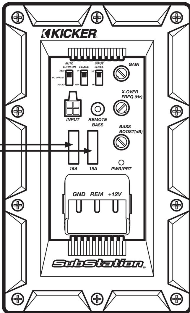
**Automatic Turn-On Selection:** KICKER powered enclosures offer three different automatic turn-on modes that can be selected on the side panel; +12V, DC Offset, and Audio. Using either the DC Offset or Audio mode causes the REM terminal to have +12V out for turning on additional amplifiers.
