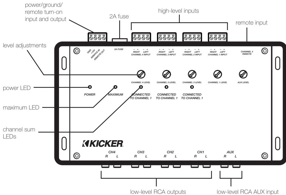
**Channel 3 Signal Sense:** If no signal is present at the Channel 4 input, the signal connected to the Channel 3 input will be routed to both the Channel 3 and Channel 4 outputs.
