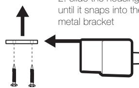
2. slide the housing until it snaps into the metal bracket
