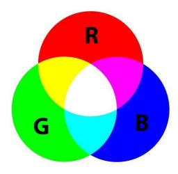
To obtain various colors of LED light (other than the 3 standard LED colors), you will need to combine 2 or 3 of the LED colors and/or vary the brightness of any of the three standard LED colors. With the 3 common standard LED colors you can produce a diverse spectrum of visible light.
