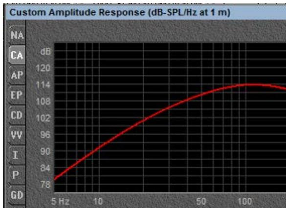
Frequency response of the same woofer in different types of enclosures with one watt of power.
