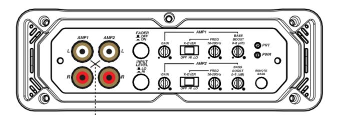
Below is an example of our 48KMA6006 6-channel amplifier. Since this amplifier is a 6-channel amp, there are two input switches rather than one. These are the "AMP2 INPUT" and "AMP3 INPUT" switches. We labeled these switches differently because this is a marine amplifier and you may not be using them with standard front/rear inputs with fader capability, you may be using "ZONE 1," "ZONE 2" and "ZONE 3" inputs instead. Despite the different labels, the buttons have the exact same function.
