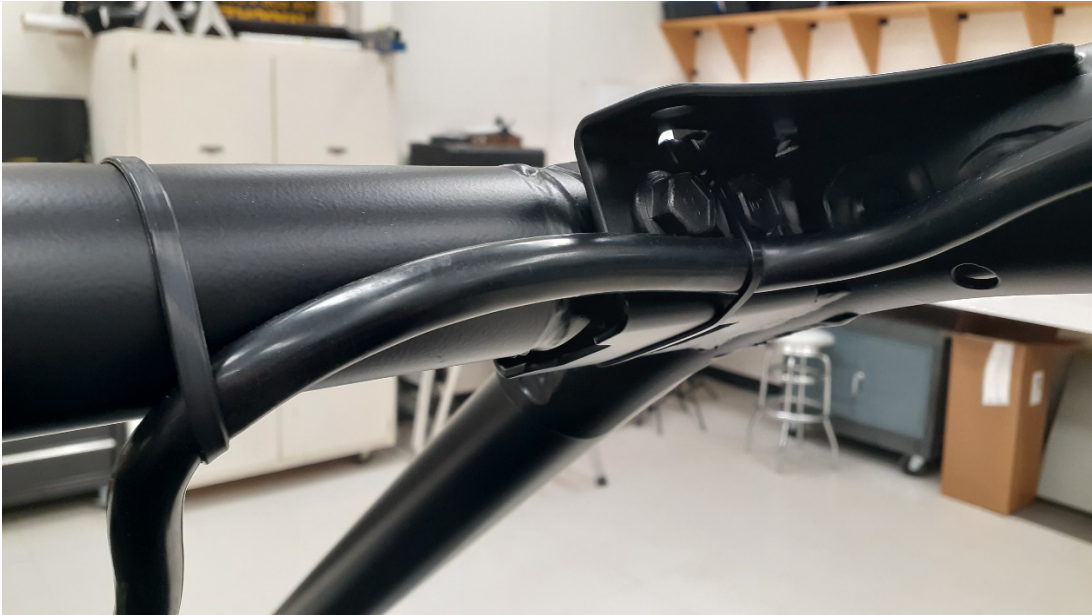
Wiring fastened with wire ties inside rollbar perimeter.
