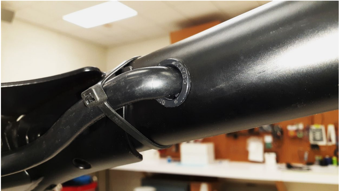
Wires entering bar through factory hole with added grommet.
