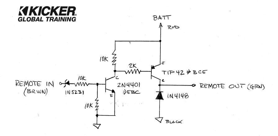
This schematic can be used for amplifing the trigger output of the Sum8 to provide enough current to drive an external relay.
