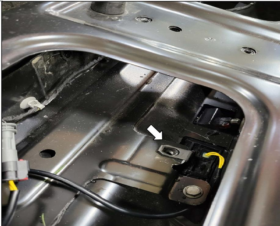
6. Install the supplied threaded clips. Fig 4
