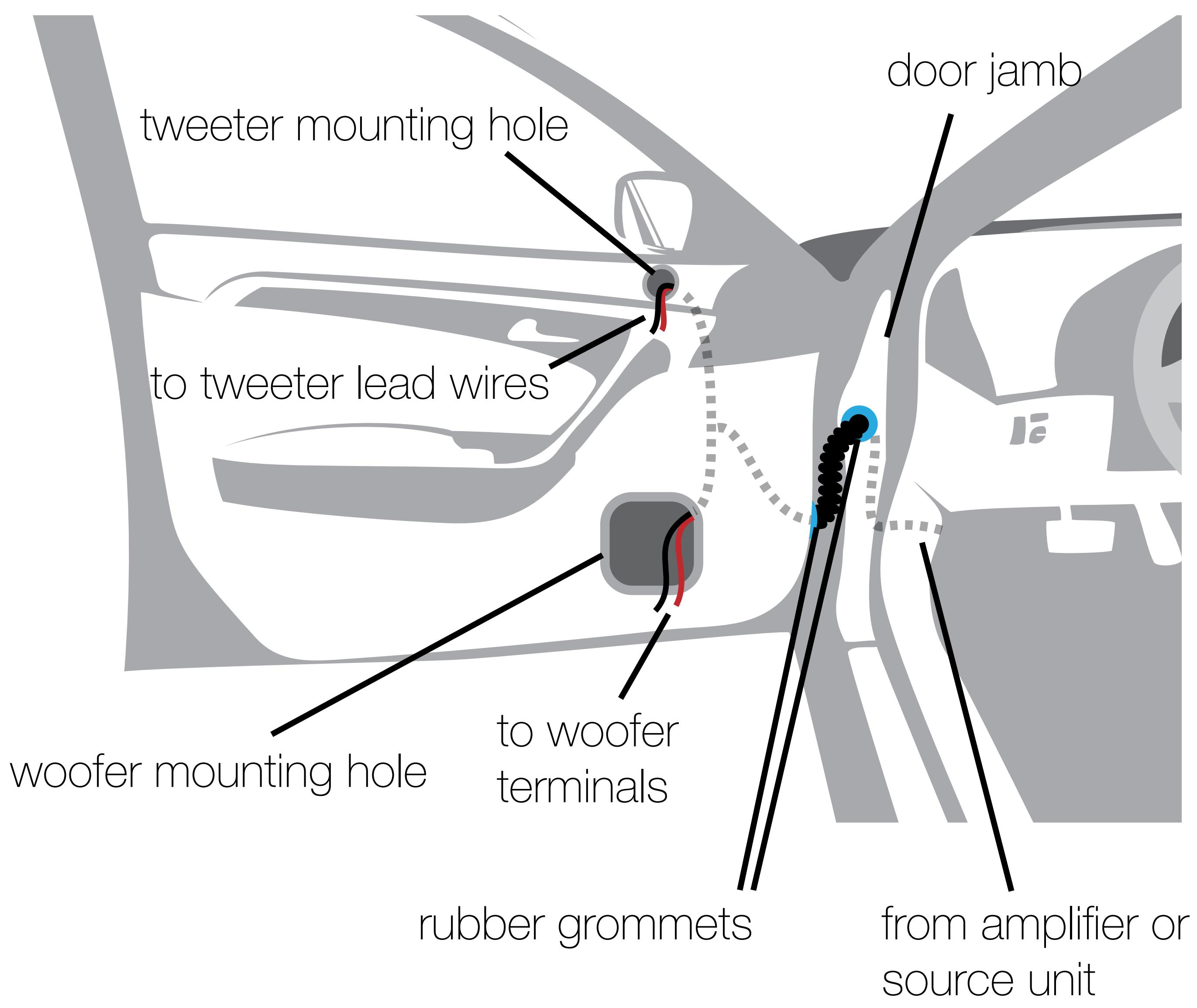
If the speaker cut-out locations require you to cut metal, avoid structural metal and braces. If the door body and panel cannot support the weight of the speaker, an optional reinforcing ring made of suitable material may be fastened or adhered to the door body.
