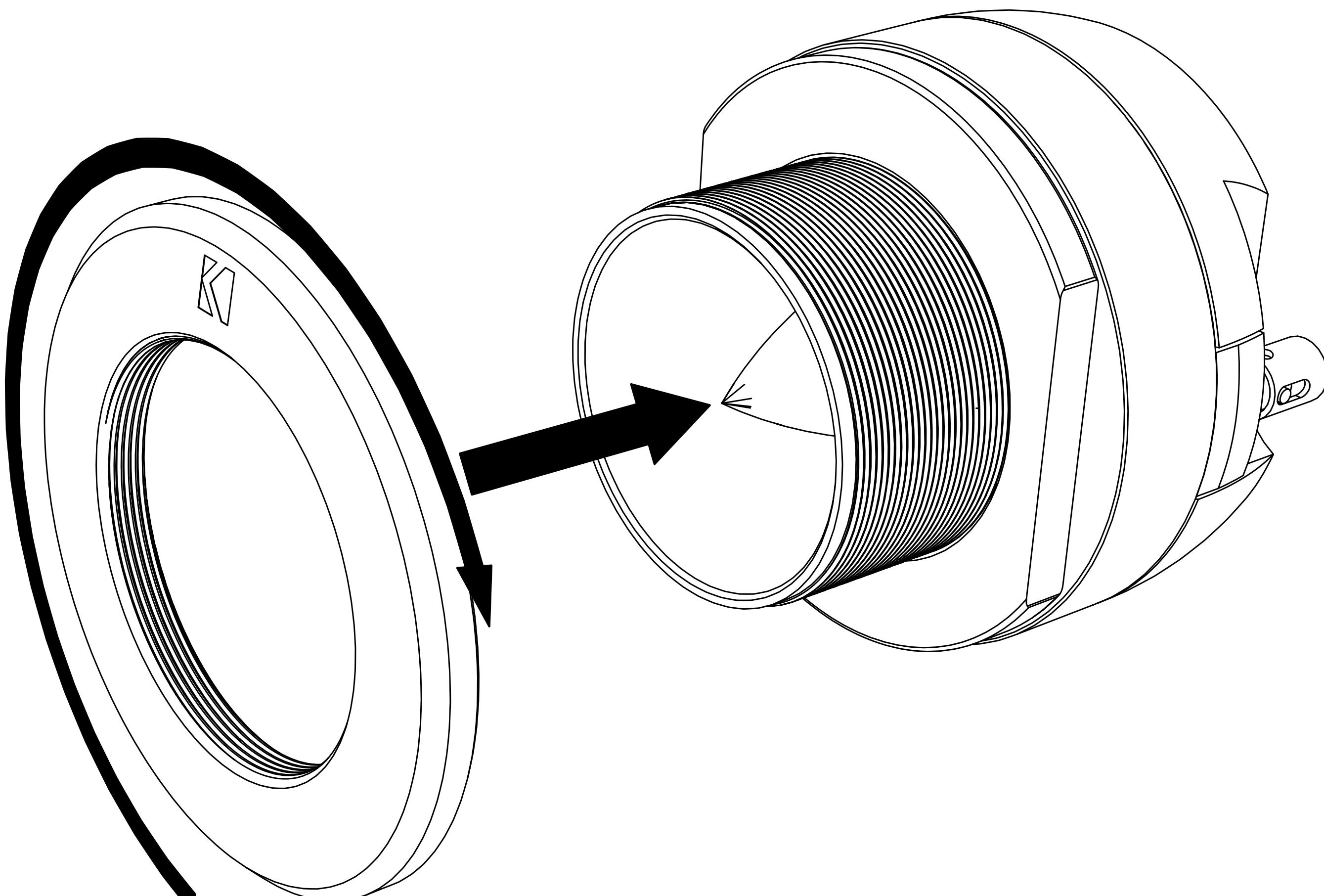
Tighten the Backing Nut towards the mounting surface to secure the Tweeter.
