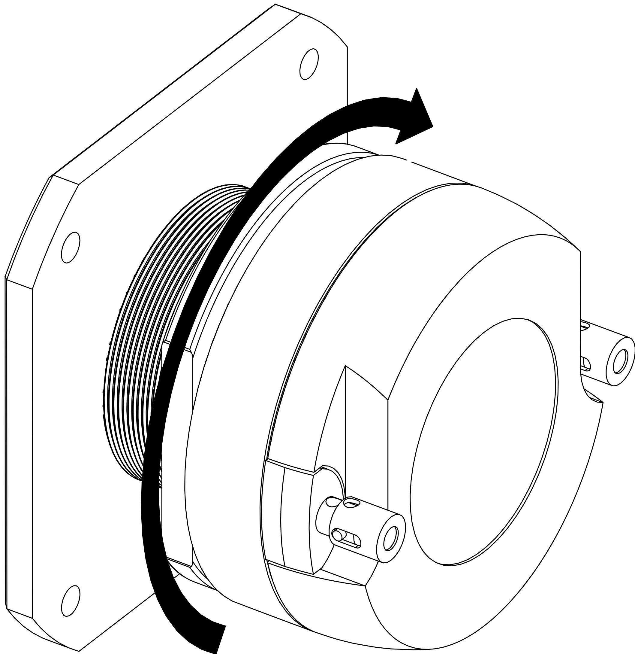
Place the Tweeter in the Mounting Hole and after finding the desired orientation, mark the mounting screw holes to be drilled by a 7/64" (2.5mm) drill bit. Secure the Tweeter to the surface using the provided screws.
