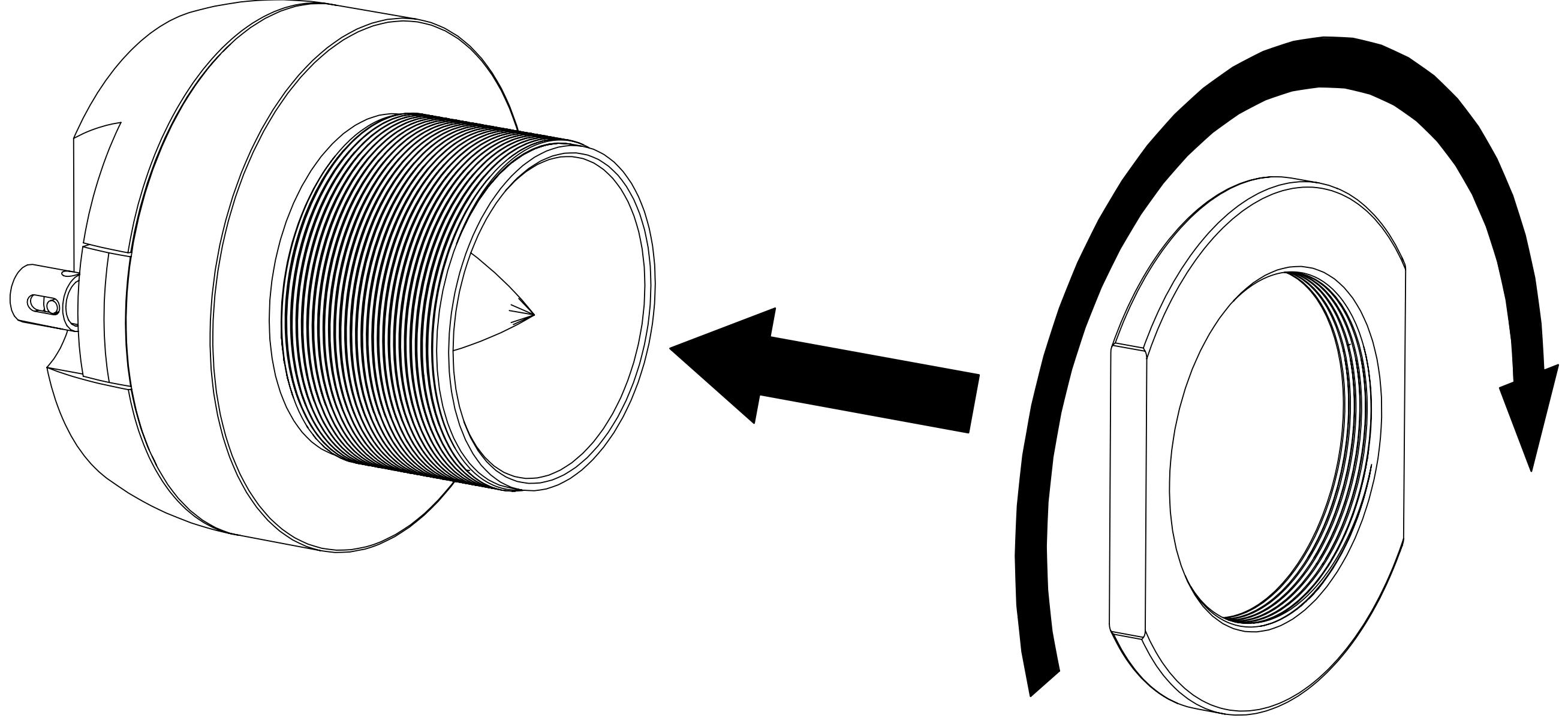
Install the Square Mounting Flange onto the Tweeter, orienting the tweeter and flange as desired.
