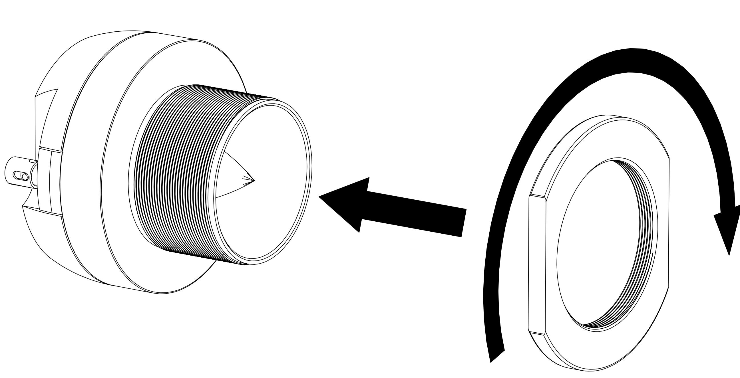
Place the tweeter in the mounting hole and install the Round or Square Mounting Flange onto the Tweeter, orienting the tweeter and flange as desired.
