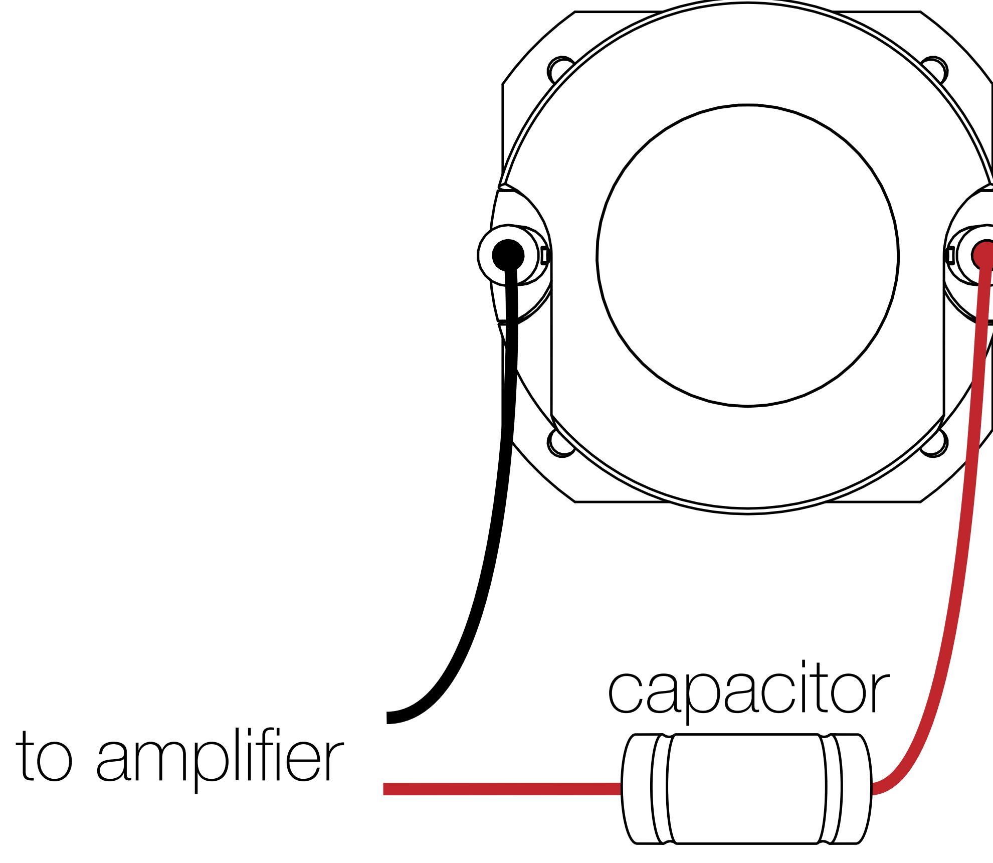
If the tweeter output is too loud, install the capacitor and resistor in series with the tweeter's Positive speaker input wire as shown.
