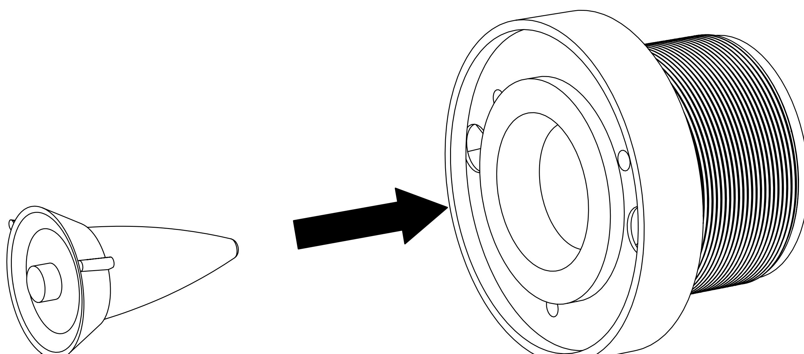
Install the motor house assembly into the horn assembly, making sure the three screw holes for both are aligned.
