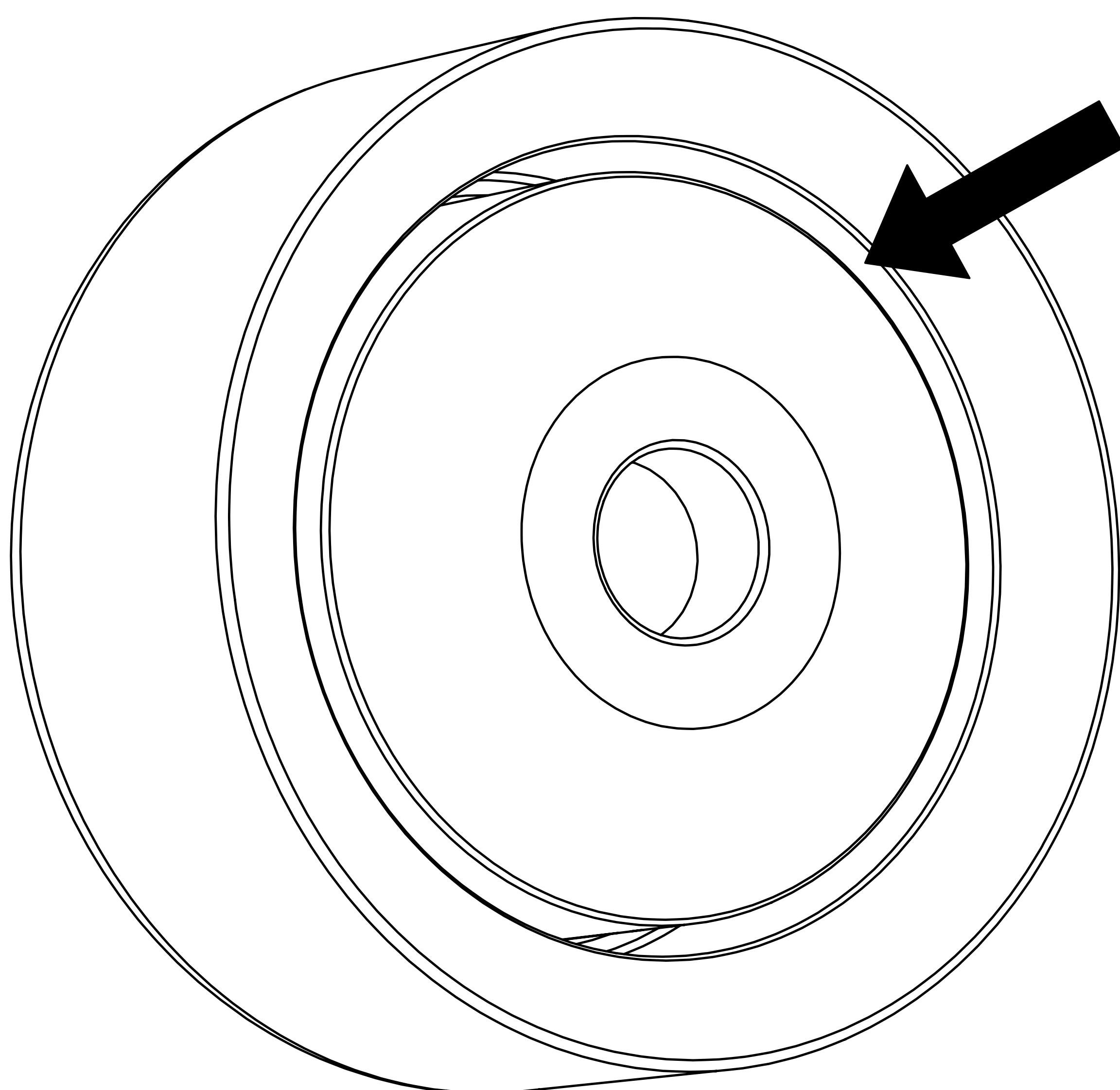
Install the back plate, washer, and motor magnet into the motor housing. Make sure the magnet is inserted with the voice coil gap out.
