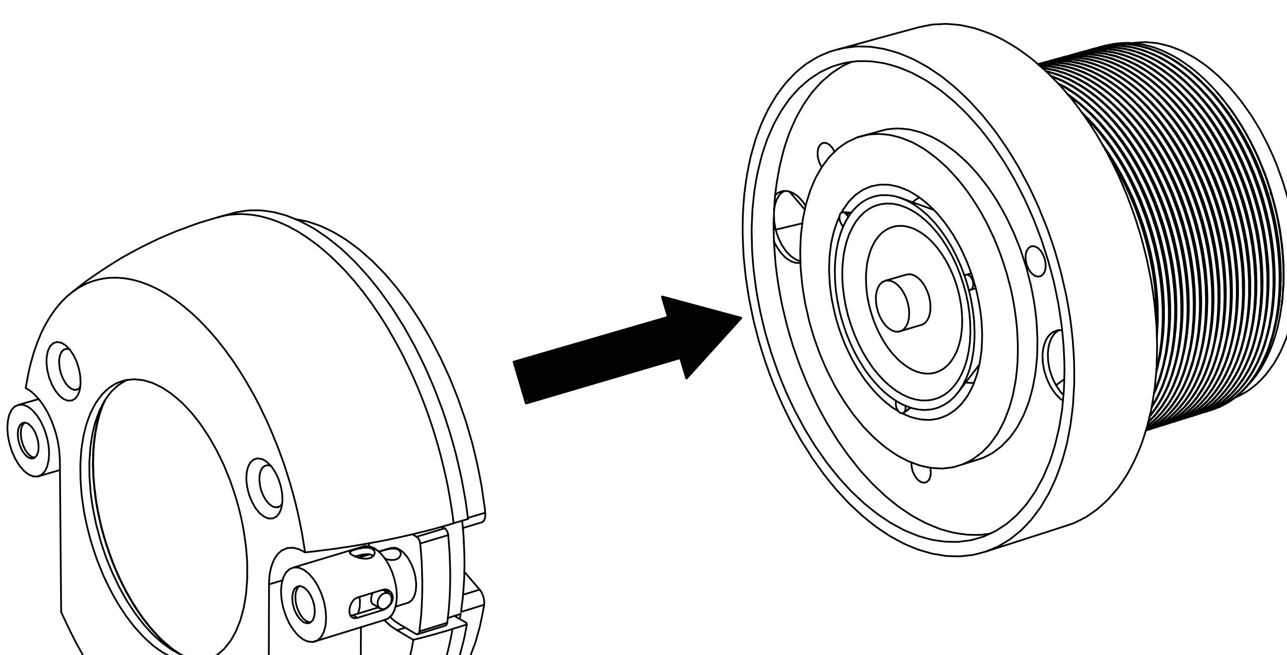
Insert and tighten the three screws.
