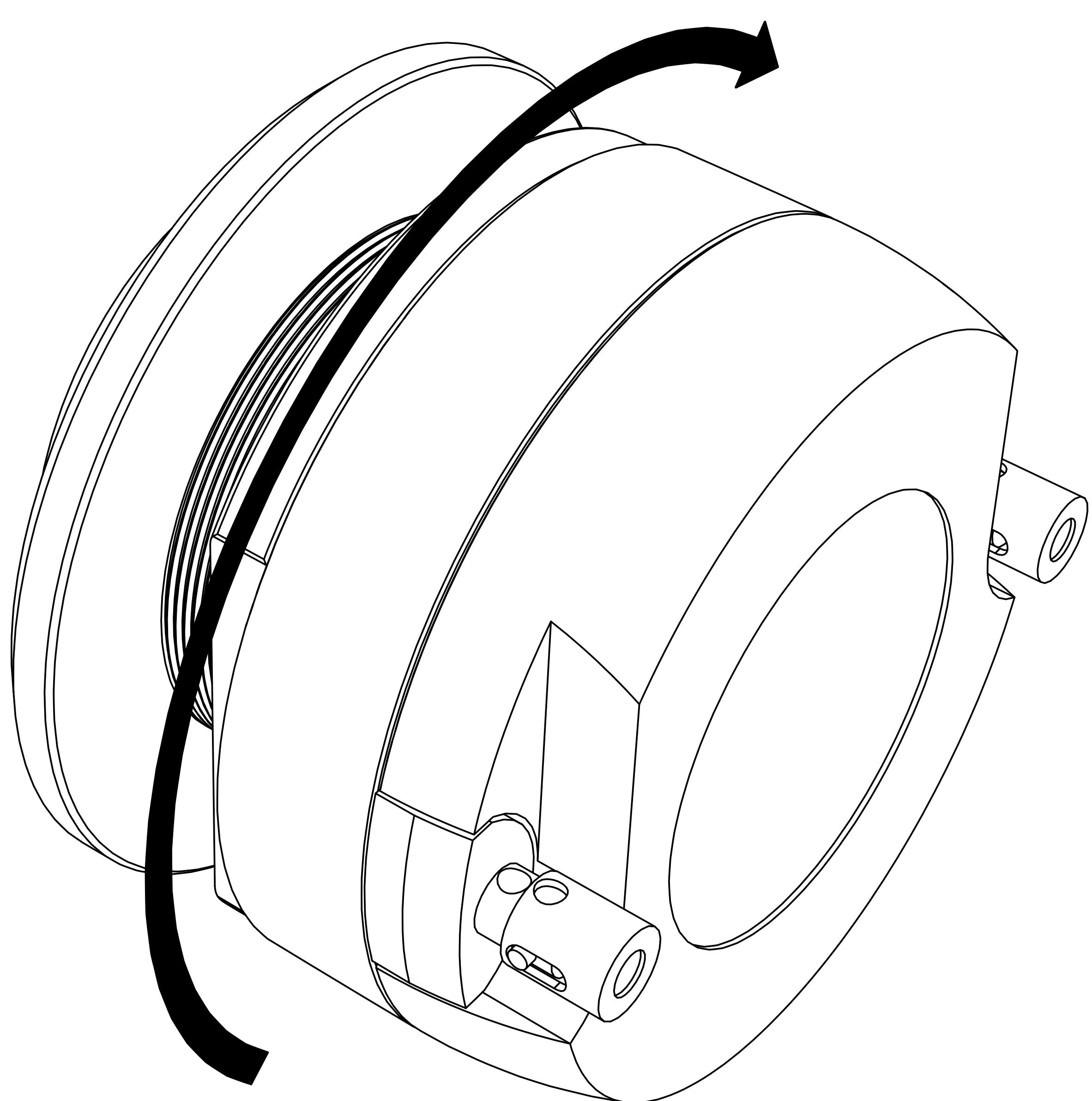
For **Surface-Mounting**, cut a circular hole in the mounting surface at 2.375" (60mm) for the ST3TW, and 3" (75mm) for the ST4TW.
