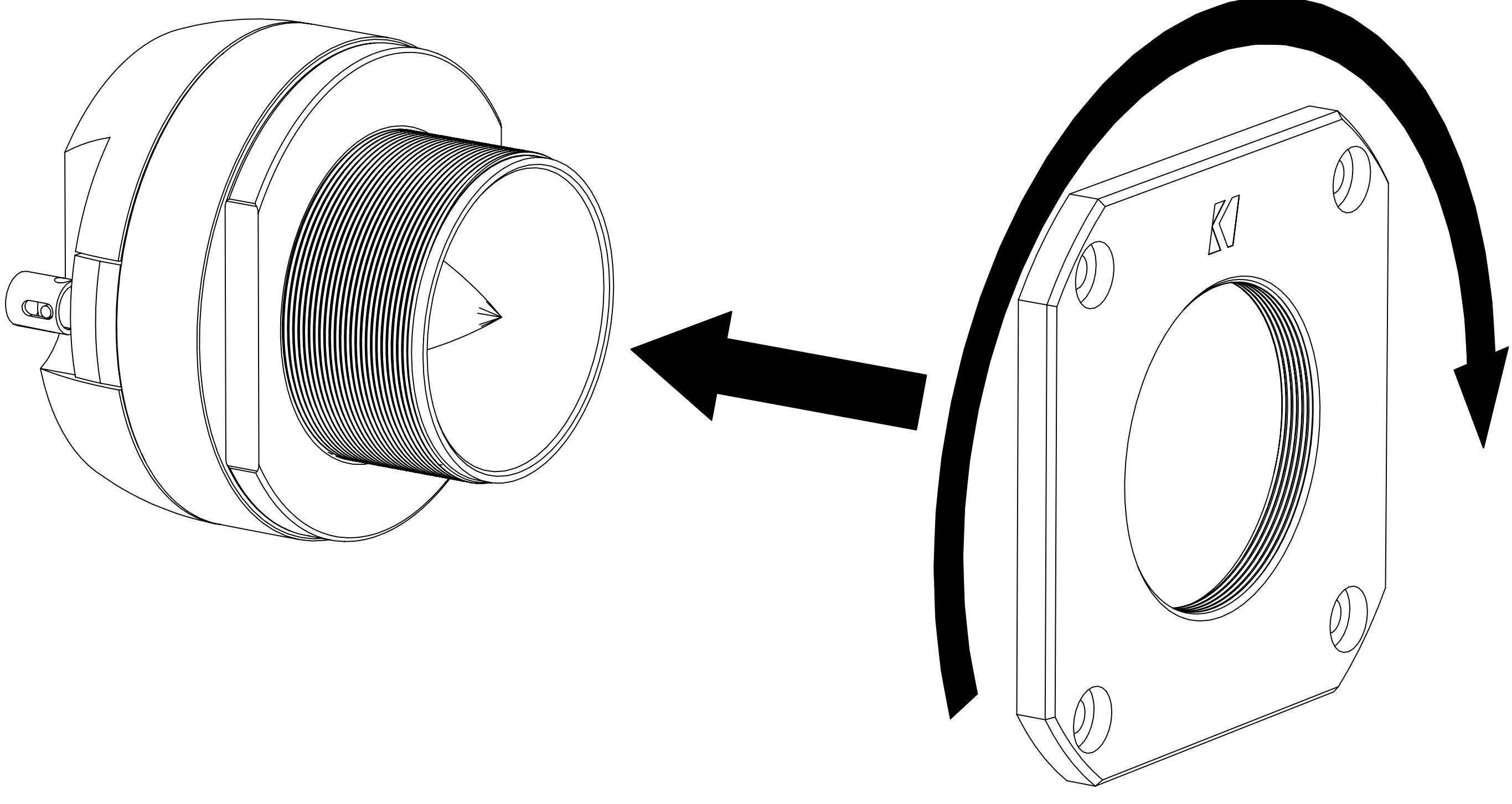
Tighten the Backing Nut to lock the Square Mounting Flange in place.
