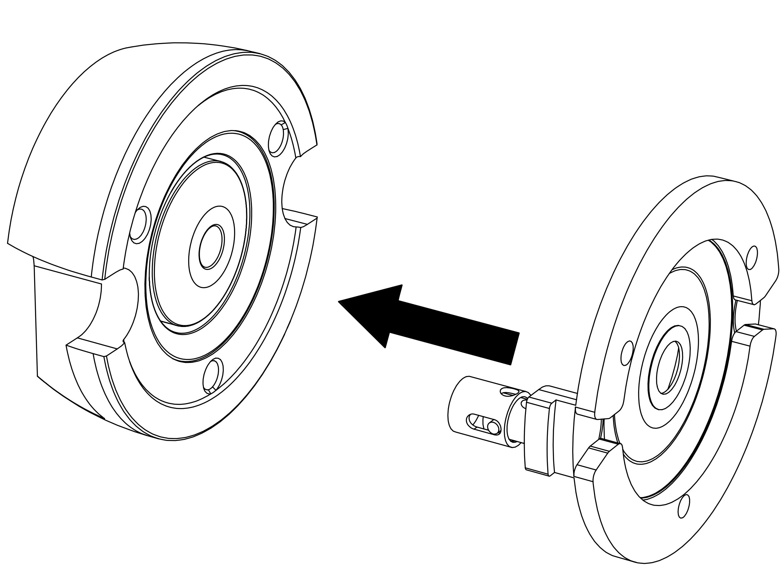
Insert the phase plug into the horn.
