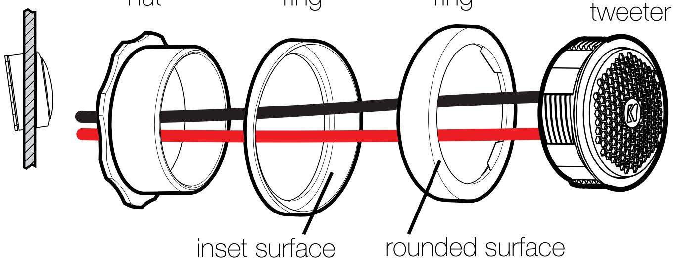
Use a 1/8 turn with tweeter tool to secure the tweeter to the mounting nut.
